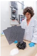
Picture 1: Processing of hybrid nonwovens from recycled carbon fibers and thermoplastic matrix fibers © A3 / Christian Strohmayer
